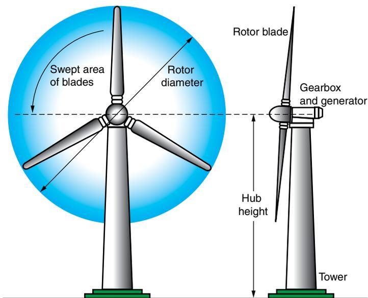
As wind turbine blades rotate, they spin a shaft, which is connected to an electrical generator. Wind turbines include a gearbox to increase the spinning shaft's speed from about 30 to 60 revolutions per minute (rpm) to the 1,000 to 1,800 rpm required by most generators to produce electricity. The hub height of most land-based turbines ranges from 60 to 100 meters. Rotor diameters can exceed 120 meters.
